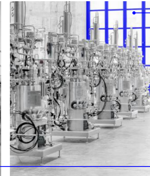
Microbial cultivation. Plant consisting of twelve 30L NLF and seven production fermenters 210L.
