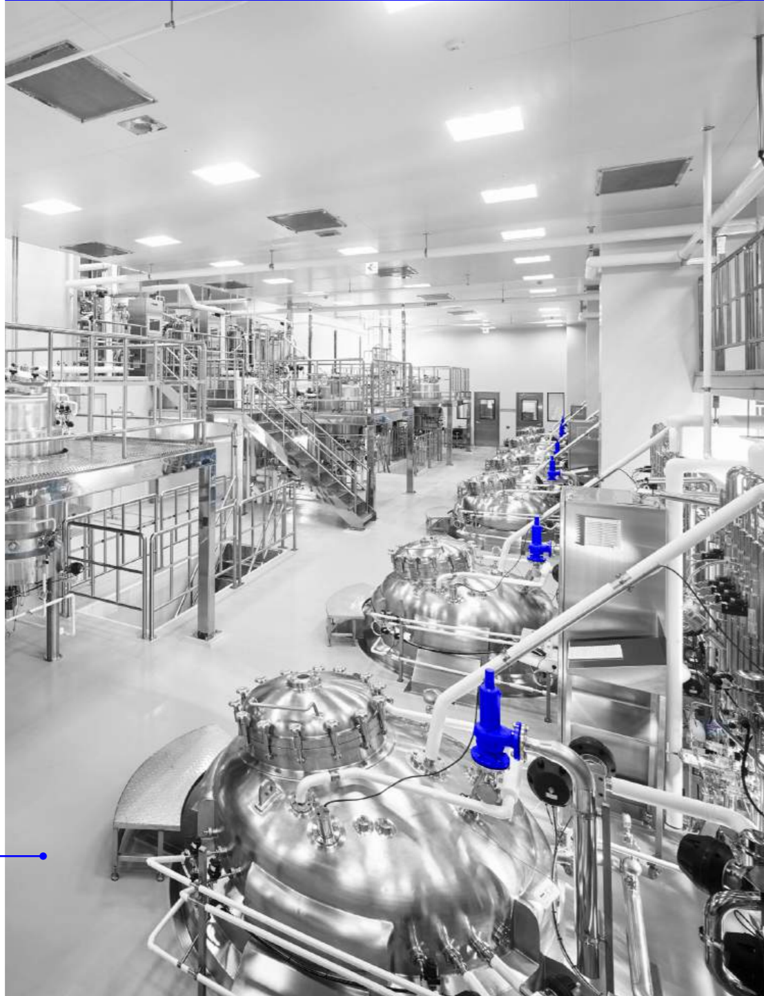
Multi-purpose cell culture production facility with five seed trains, each with 120L, 600L and 3,000L bioreactor systems, and two 15,000L production bioreactors per train.
