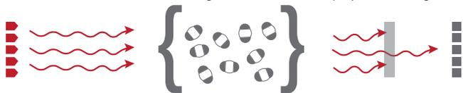
If CO<sub>2</sub> levels are high, a lower number of IR rays pass through.
