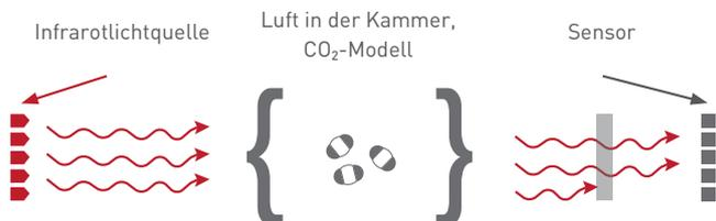
If CO<sub>2</sub> levels are low, a high number of IR rays pass through.
