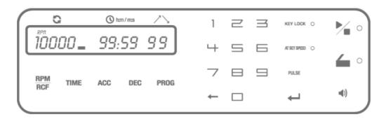
□ RPM/RCF For automatic conversion of RPM/RCF and to set the speed
