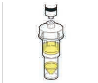
2 Place the cell cap onto the retentate cell and gently screw into place. Pressurize the unit by injecting 10 ml of air with a syringe.
